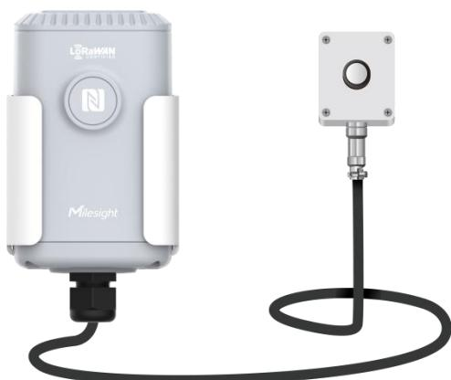
EM500-LGT is designed for measuring light in harsh environments and transmitting data using LoRaWAN® technology. With this low power consumption technology, EM500-LGT can work up to 10 years with 19000 mAh battery. Combining with Milesight LoRaWAN® gateway and Milesight IoT Cloud solution, users can manage all sensor data remotely and visually.
