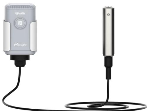
EM500-SWL is designed for measuring liquid level in harsh environments and transmitting data using LoRaWAN® technology. With this low power consumption technology, EM500-SWL can work up to 10 years with 19000 mAh battery. Combining with Milesight LoRaWAN® gateway and Milesight Development Platform solution, users can manage all sensor data remotely and visually.
