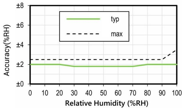
3. Typical RH accuracy corresponding to the temperature:
