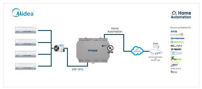
Figure 4. Integration of Midea AC systems into Home Automation installations
