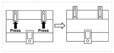
2. Use the clip holes to fix the gateway on the wall using screws.
