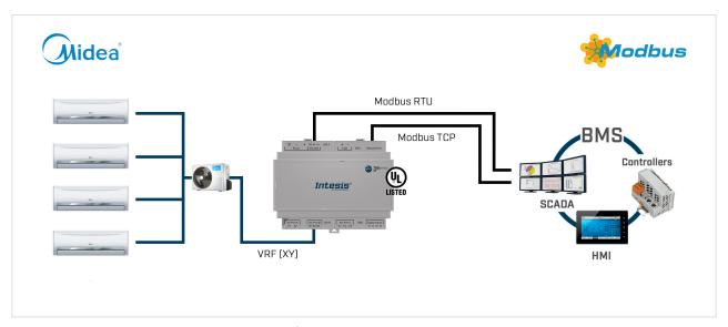
Figure 1. Integration of Midea AC systems into Modbus installations
