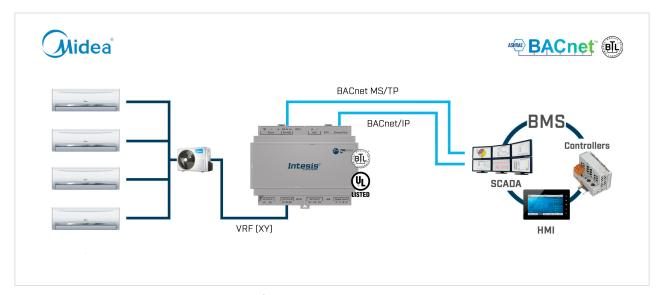
Figure 2. Integration of Midea AC systems into BACnet installations
