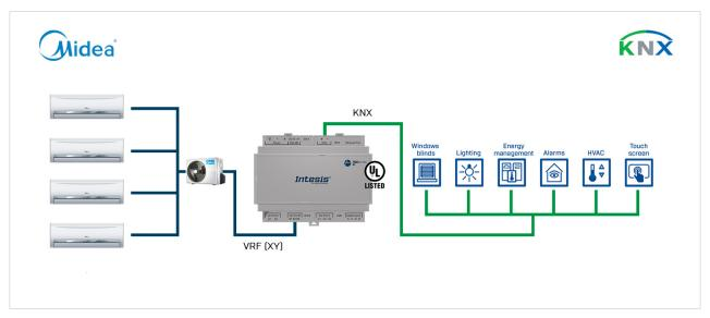
Figure 3. Integration of Midea AC systems into KNX installations
