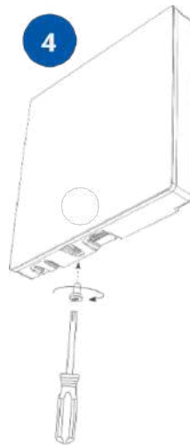
Figure 18. Screw the panel to the back box
