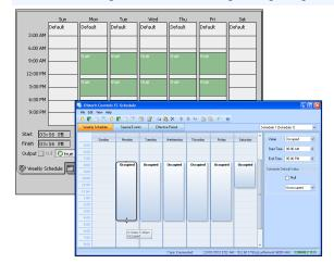
Configure the controller's built-in schedules and holidays from the EC-Net<sup>AX</sup> solution (ECB and ECL series controllers), LNS (ECL series controllers), or directly from within EC-*gfx*Program (ECB and ECL series controllers) with an easy-to-use point, drag, and click interface. It features a weekly schedule for regular, repeating, events by "time-of-day" and "day-of-week", while a holiday schedule is available to define events for specific days.
