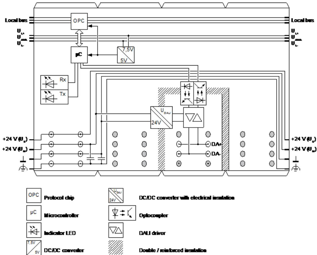
Figure 1 Internal wiring of the terminal points
