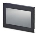
Touch panel with 17.8 cm/7" TFT-display (analog resistive (polyester)), 800 x 480 pixel(s) (WVGA), 16.7 million colors, i.MX 6DualLite, 454 MHz, 1x USB Host 2.0, 1 x Ethernet (10/100 Mbps), RJ45, Yocto/Linux and user software: QT browser. (bus system: without)
